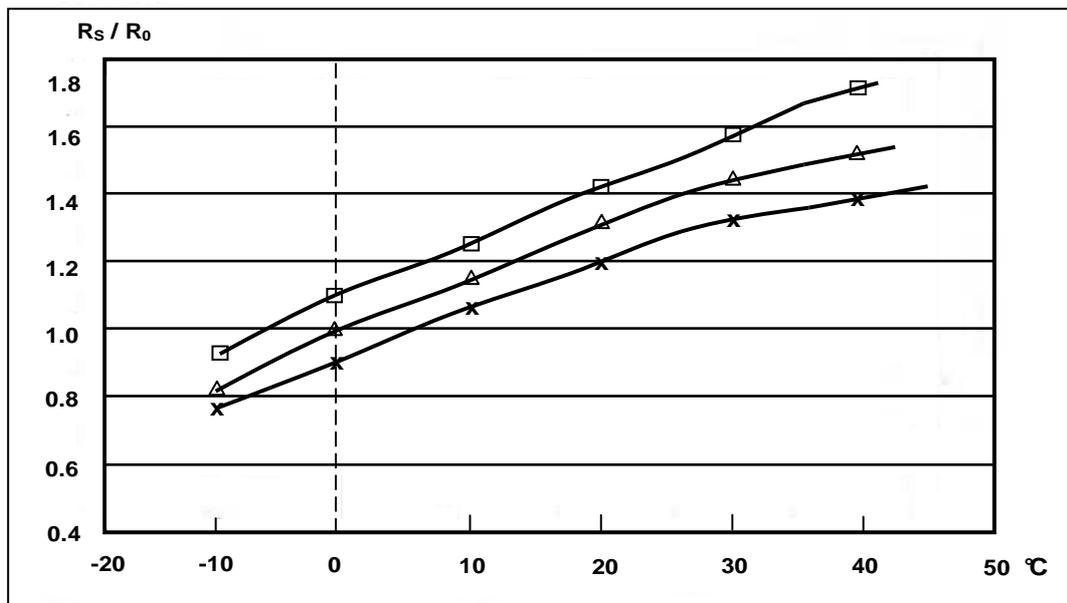
**Figure 2b.** Relation between surface resistance of HS-135 with environment related temperature
