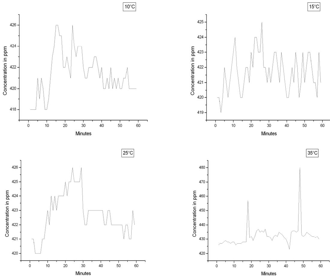
**Figure 5.** Variations in the rate of CO<sub>2</sub> as a function of temperature
