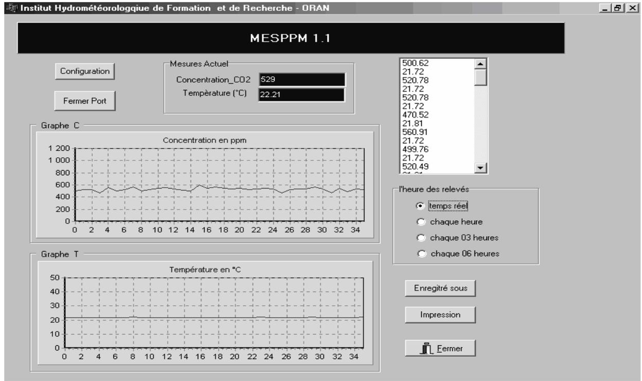
**Figure 4.** The Graphical User Interface (GUI) of acquisition and restitution of CO<sub>2</sub> data
