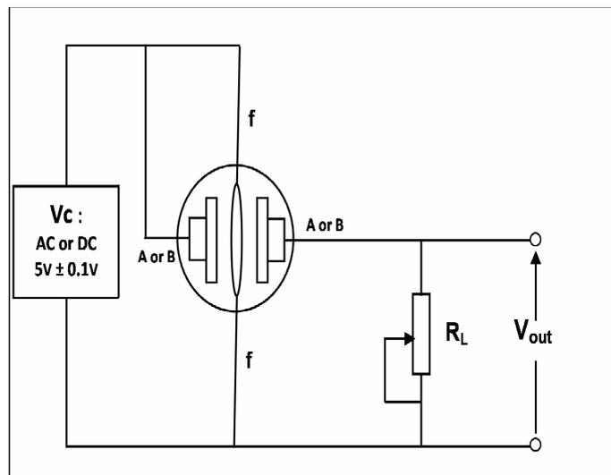
**Figure 1.** Standard test circuit of HS135 [12]
