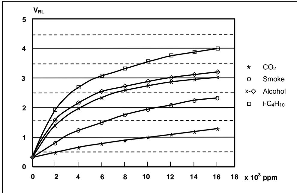
**Figure 2a.** Relation curve of V<sub>RL</sub> and gas concentration
