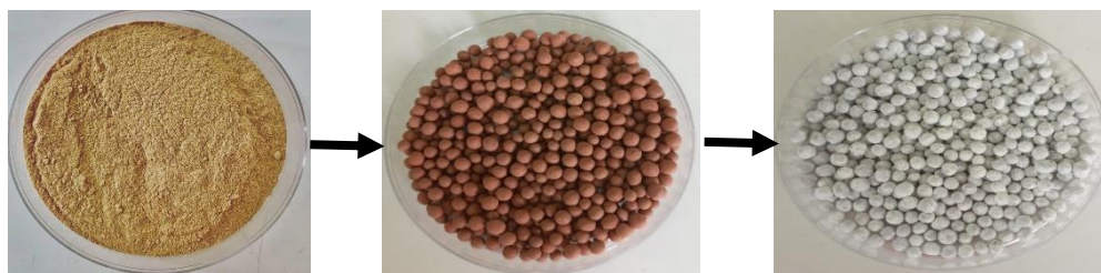
Figure 2: Preparation steps of the supported photocatalyst (clay-TiO 2 )
