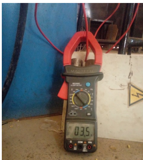
Figure 2. Experimental setup using clamp meter to measure current
