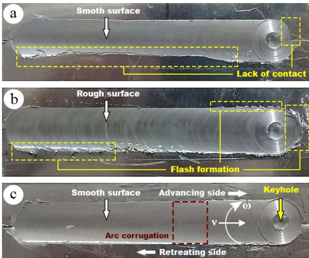
**Figure 2.** Surface appearance of the FSW samples at tool rotation speed of 600 rpm and tool travel speeds of (a) 45, (b) 60, and (c) 75 mm/min.
