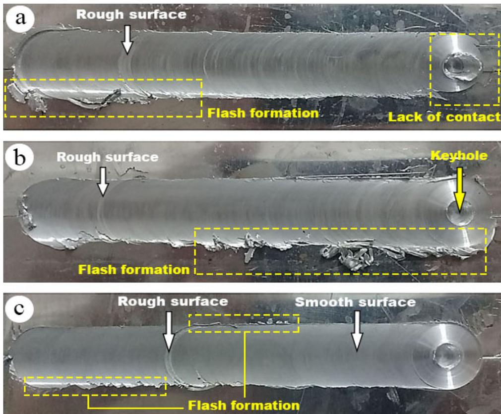
**Figure 1.** Surface appearance of the FSW samples at tool rotation speed of 400 rpm and tool travel speeds of (a) 45, (b) 60, and (c) 75 mm/min.
