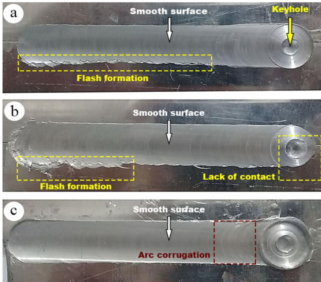
**Figure 3.** Surface appearance of the FSW samples at tool rotation speed of 800 rpm and tool travel speeds of (a) 45, (b) 60, and (c) 75 mm/min.
