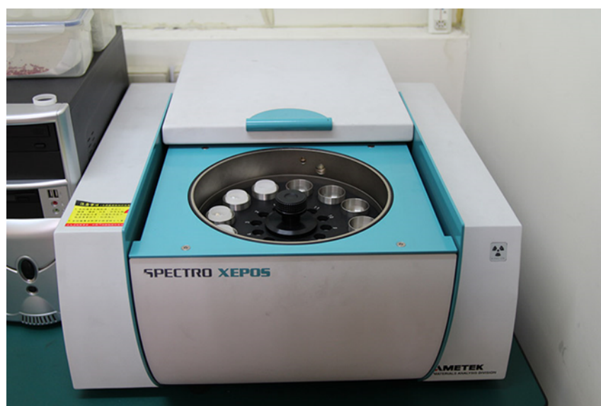
Figure 2 : The X-ray fluorescence spectrophotometer SPECTRO XEPOS
