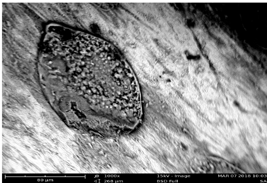
Figure 3b Scanning Electron Microscopy of Mild steel with 0.5 M Hydrochloric acid with Euphorbia heterophylla
