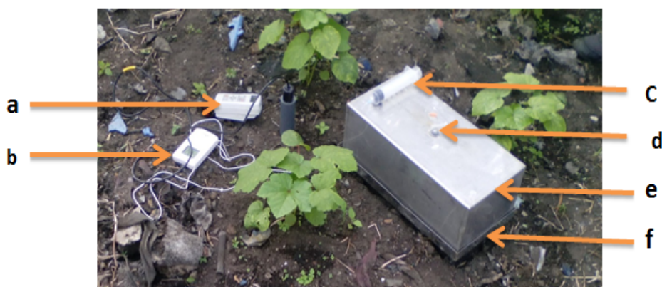
Fig. 2: Equipment used in the flux chamber measurements. a: soil moisture probe; b: air and soil temperature probe; c: syringe; d: septum (sampling port); e: chamber (length=40 cm * width=20 cm * height=18 cm); f: chamber frame inserted into the soil.
