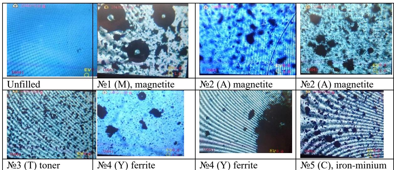
**Figure 3:** Optical microphotographs of epoxy compositions with magnetites, with an increase of 100 times (with a screen base length of 7 cm).
