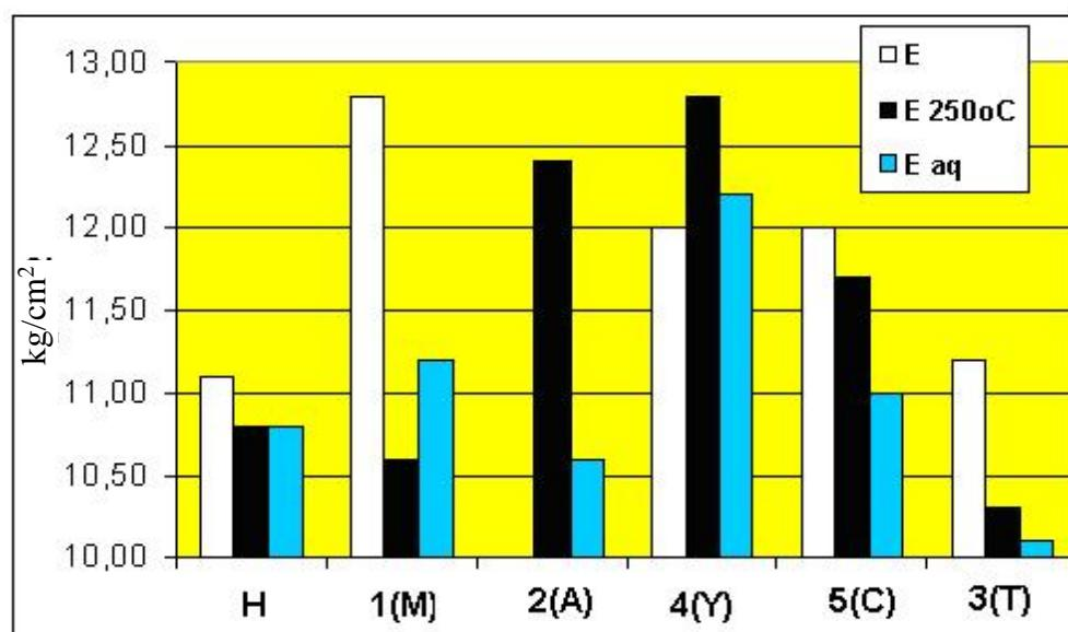
**Figure 6:** A comparative histogram of the values of the modulus of elasticity of compression of the samples at different exposure modes - the usual 60 °C; hard 250 °C and exposure in water for 7 days (Eaq).
