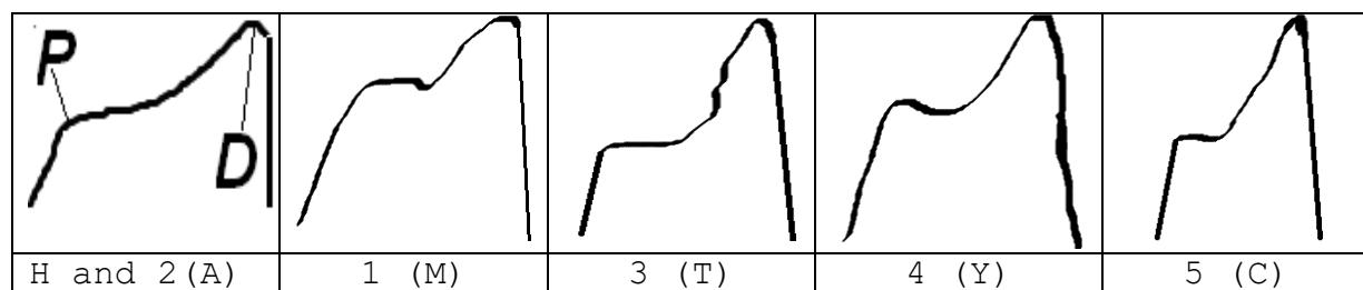
**Figure 5:** The type of compression diagram «load-deformation » for different composites, after conventional heat treatment (50-60 °C).
