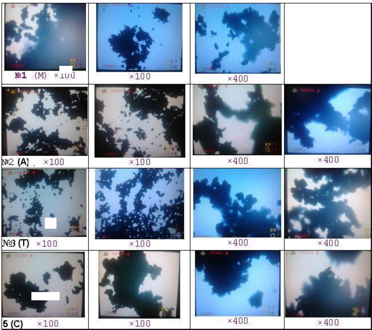
**Figure 2:** Optical microphoto of magnetite powders, with an increase of 100 or 400 times (with a screen length of 7 cm).
