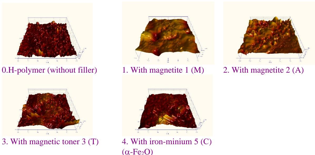
**Figure 1:** AFM images of the surface of composites
