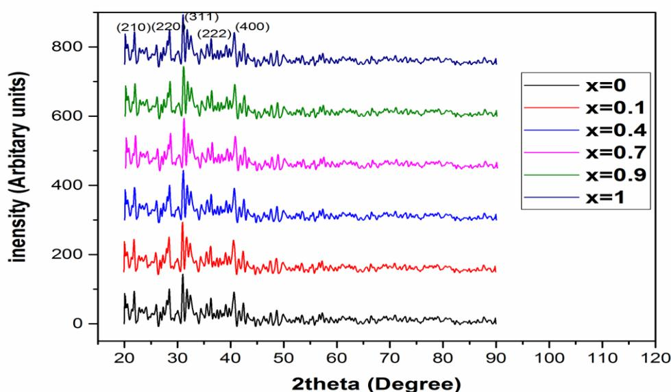
Figure 1: X-rays diffraction pattern of  $\text{Co}_x\text{Zn}_{1-x}\text{Fe}_2\text{O}_4$
