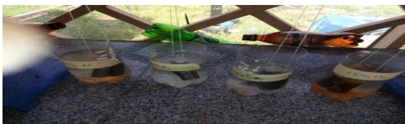
Figure 5: The samples immersed in the environment (Seawater)
