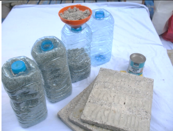
Figure 1: Gathering the brick's constituents – filled containers, precast concrete plates and the glue
