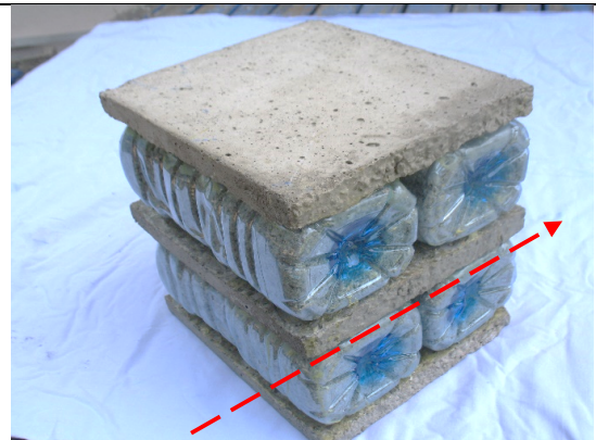
Figure 6: The brick can be used as a slab element when disposed of horizontally, along (z) axis showed as red dashed line
