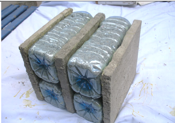
Figure 5: Bonding the third concrete plate with the second insulating layer to obtain the whole brick
