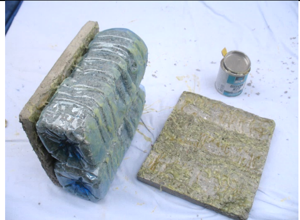
Figure 2: Bonding two containers with the first concrete plate to form the first insulating layer
