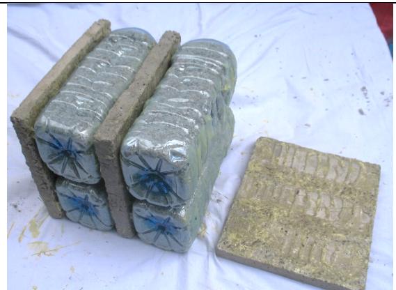
Figure 4: Adjusting and bonding the second insulating layer with the second concrete plate
