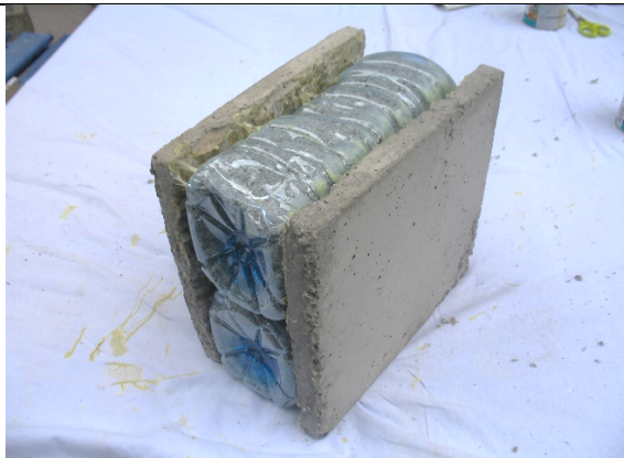
Figure 3: Bonding the second concrete plate with the insulating layer, which has to be all adjusted
