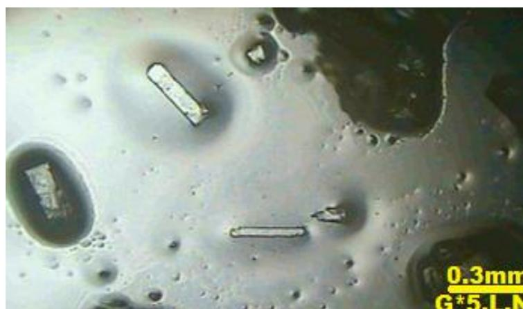
**Figure 2.** Photograph of a grown crystal of PABADHP.
