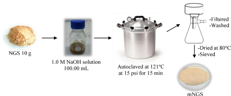
**Figure 2:** Schematic for biosorbent preparation.
