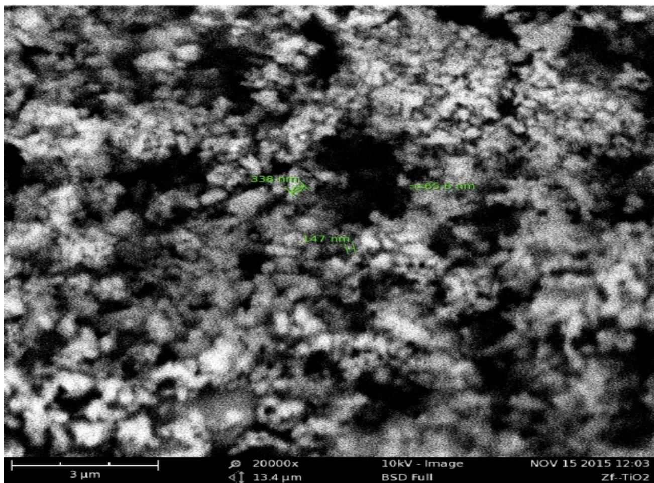
**Figure 2:** SEM image of the ZnFe<sub>2</sub>O<sub>4</sub>-TiO<sub>2</sub> nanocomposite
