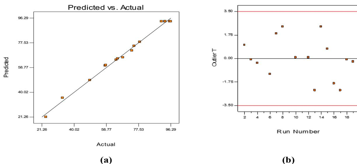
**Figure 3:** Diagnostic plots for photocatalytic mineralization of acetaminophen showing (a) actual vs. predicted values of photocatalytic mineralization of acetaminophen, and (b) internally outlier T points.
