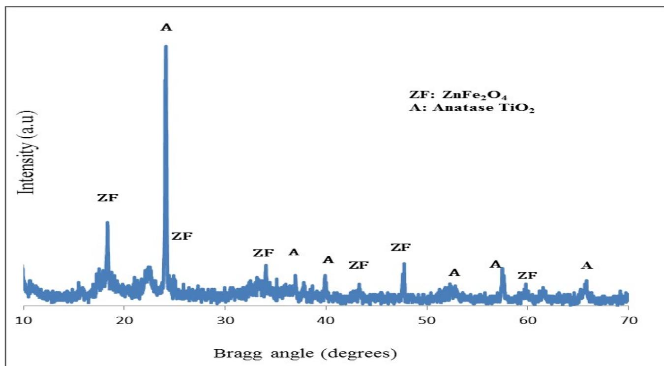
**Figure 1:** XRD pattern of the ZnFe<sub>2</sub>O<sub>4</sub>-TiO<sub>2</sub> nanocomposite
