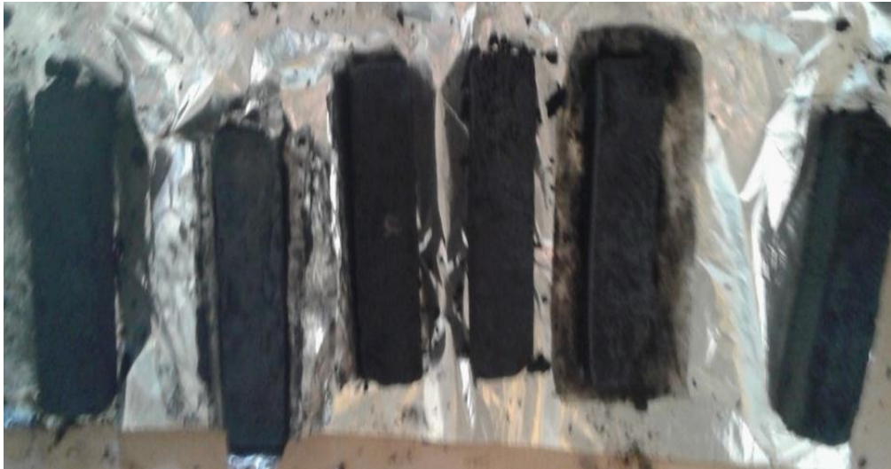
Figure 9.a: A view of specimens with raw and treated PG-TPT- based material
