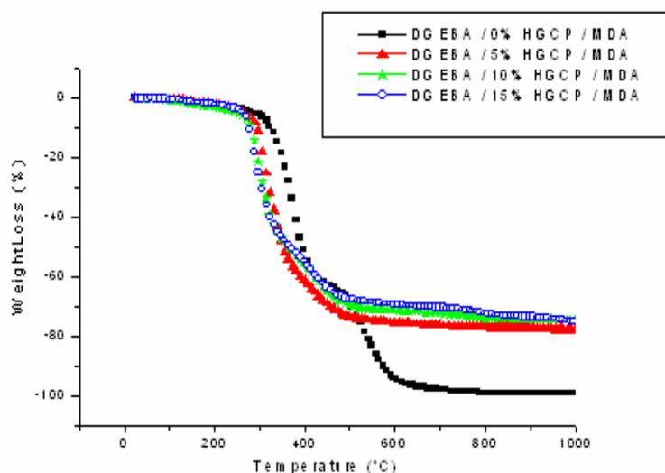
**Figure 2:** TGA thermogram of samples: (DGEBA/0%HGCP/MDA), (DGEBA/5%HGCP/MDA), (DGEBA/10%HGCP/MDA) et (DGEBA/15%HGCP/MDA). Analysis under in  $N_2$  atmosphere at a  $10^\circ C \text{ min}^{-1}$  heating rate.
