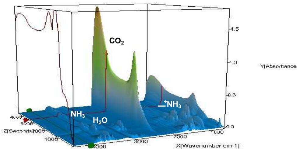
**Figure 4:** FT-IR spectrum of gas evolved during TGA of sample (DGEBA/HGCP/MDA) in air atmosphere at a  $10\text{ }^{\circ}\text{C min}^{-1}$  heating rate.
