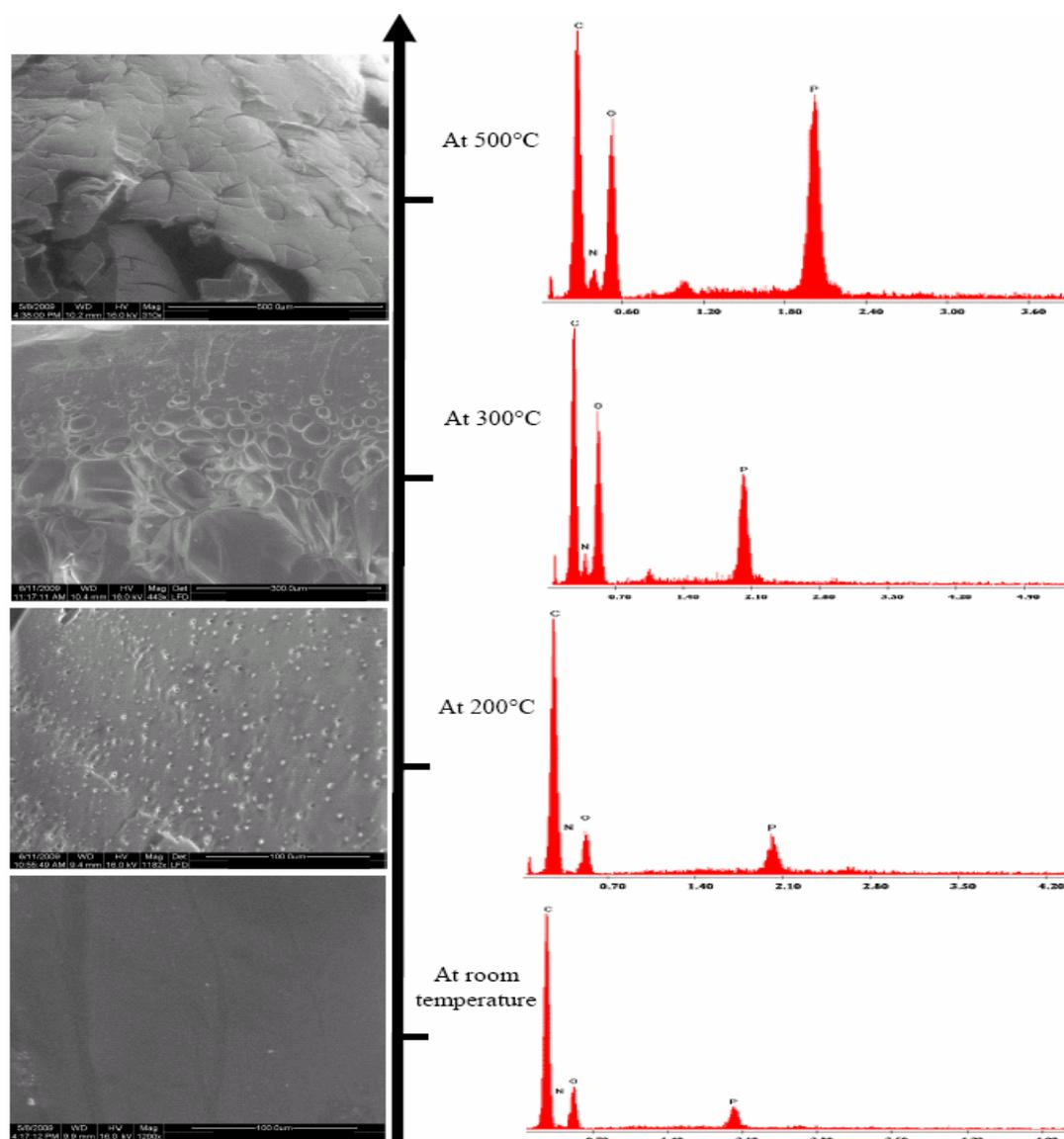
**Figure 3:** SEM images of inflammable gas evolution and char formation process for intumescent protection of burned specimen of (DGEBA/HGCP/MDA) and its EDX analysis.
