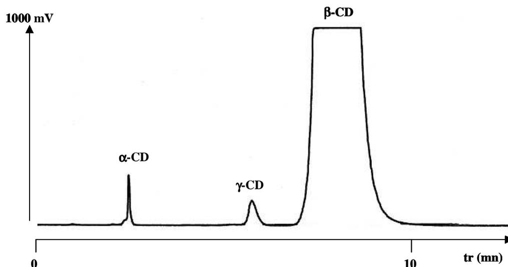
Figure 4b: Isocratic analysis of  $\alpha$ -,  $\beta$ - and  $\gamma$ -CDs with gain 16
