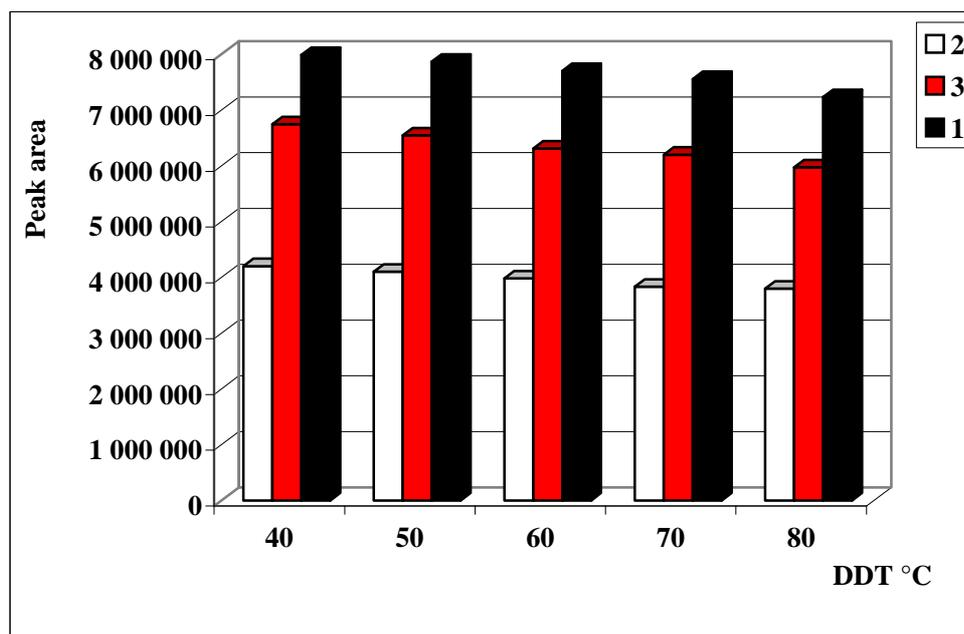
**Figure 2:** Effect of DTT of ELSD on the response of  $\alpha$ -CD (1),  $\beta$ -CD (2) and  $\gamma$ -CD (3)
