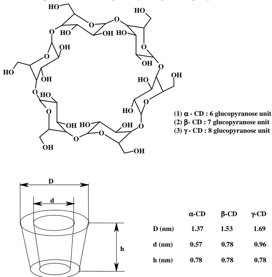
**Figure 1:** Chemical structures and molecular dimensions of  $\alpha$ -,  $\beta$ - and  $\gamma$ -CDs
