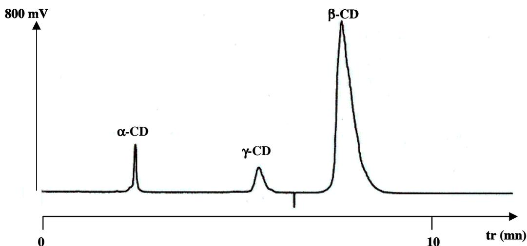
Figure 4c: Isocratic analysis of  $\alpha$ -,  $\beta$ - and  $\gamma$ -CDs with gain 8 and 16
